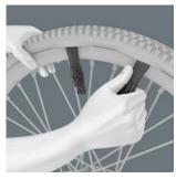
With the glass fibre reinforced plastic tyre jacks, the tyres can be safely levered off the rim without damaging the rim. Lift off of the rim with one tyre jack, hook into a spoke and pull off the tyre with the second tyre jack. The two tyre jacks can be clicked together and are therefore not lost individually.
