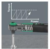
The Safe-Torque A2 torque wrench is equipped with a slide-over mechanism. Once the set torque has been reached, the tool cannot be overtightened, so that excessive torque cannot be applied.
