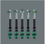
The ratchet head pivots freely and can be locked into any defined position by using the slide switch that is positioned on either side. It is even possible to work in very confined and difficult-to-access areas with enhanced hand clearance. The predefined locking at 0°, 15° and 90°, both to the right and left, ensure safe working without any slipping of the ratchet head.
