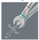
Thanks to the open end side offset by 7.5°, double hexagon geometry and an adjusted application method (placement – screwdriving – turning – turning, etc), even screwdriving challenges allowing a return angle of less than 30° can be solved.
