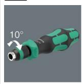
The integrated ratchet with fine toothing (36 teeth) and a return angle of 10° eases and accelerates screwdriving without having to reposition the tool.
