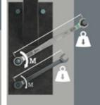
Unique combination of open end and ring ratchet mechanism in a long design. The long lever allows for higher power transmission. The long design also improves accessibility at low-lying couplings.
