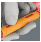
The recesses in the fast-rotating sleeve allow resistance to be generated by finger force. This allows the ratchet mechanism to be used even at low resistance of the screw.
