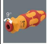
The integrated ratchet with fine toothing (40 teeth and a return angle of 9°) eases and accelerates screwdriving without having to reposition the tool.
