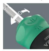
Intuitive switching of the ratchet mechanism. Turn the switch clockwise for clockwise screwdriving; turn it counterclockwise for counterclockwise screwdriving. Use position 0 to deactivate the ratchet mechanism for precise working.
