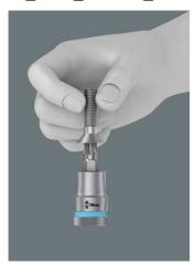
The new 3/8 "bit <u>sockets</u> from Wera feature an innovative holding function that holds screws securely on the tool. In the TORX® profile, for example, a special geometry creates a clamping force between the tool and the screw.
