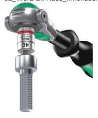
With the new In-Hex bit sockets for hexagon socket screws, the holding function is achieved by a special ball retention mechanism. After tightening the screw, the tool can be removed again without difficulty.
