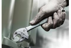
The self-setting spanner Joker 6004 automatically and continuously sets the required size when the tool is placed on the hexagon bolt or screw. By using the corner-width prisms in the front of the jaw, a return angle of only 30° can be realized, great for working in confined spaces.
