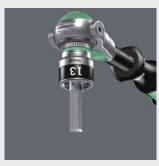
The clamping of the screw is achieved by two flexible locking balls and a robust, permanently elastic, heat-shrunk tubing. The tubing is effectively protected against mechanical wear and tear by a steel ring. The holding function is especially helpful in confined, hard-to-reach spaces, where there is no room for a second hand to secure the screw.
