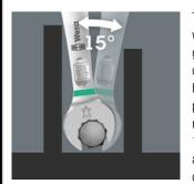
The Joker 6003 combination wrench with its special mouth geometry – an open-end offset by 7.5° and the double hexagon profile – doubles the placement possibilities when repeatedly turning the wrench 180° around the longitudinal axis. Bolts and screw heads can be "accessed" every 15°.
